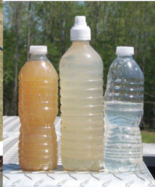
Photo: JASON SHOLTZ The bottle on the left is untreated water. The other two are treated. The one in the middle was discharged directly on riprap. The one on the right was discharged through a sediment bag, but they float to the surface.
